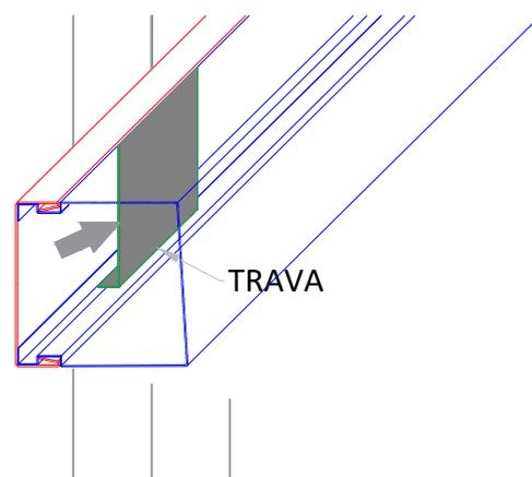
AS TRAVAS DEVEM SER DESLIZADAS POR DENTRO DA LÂMINA PARA IMPEDIR QUE DESENCAIXEM DO PORTA PAINEL. (UMA TRAVA A CADA 1,25M)
