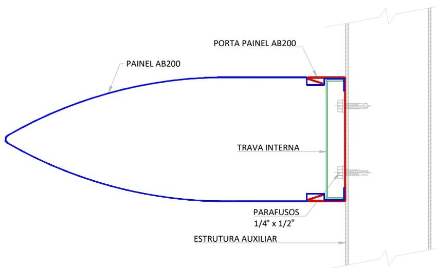
AS TRAVAS DEVEM SER DESLIZADAS POR DENTRO DA LÂMINA PARA IMPEDIR QUE DESENCAIXEM DO PORTA PAINEL. (UMA TRAVA A CADA 1,25M)
